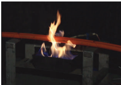
Smoke Density Test (IEC 61034)
