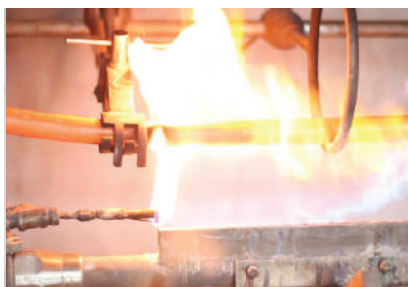
Resistance to Fire Alone Test (Category C)
